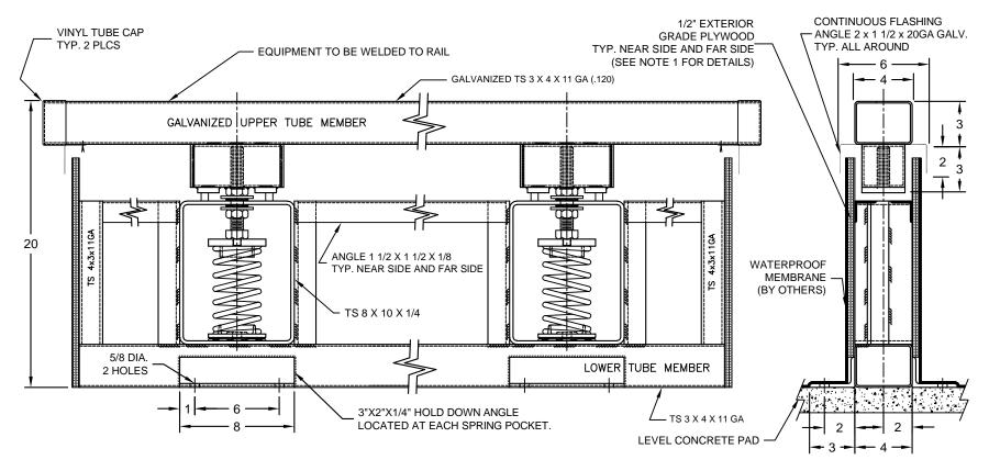
NOTE 1: ONE (1) PLYWOOD FASCIA TO HAVE CUT-OUTS MATCHING SPRING POCKET LOCATIONS. THE REMAINING FASCIA TO BE WITHOUT CUTOUTS.
